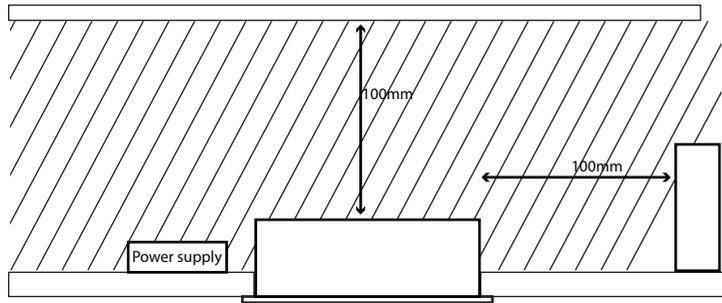
Rear of fitting may abut structural members and building elements. Do not install through or directly into joist, beam, rafter or ceiling batten.
