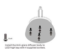
Note: Please check highbay label to see if fitting is dimmable and if so which type of dimming. Available in Non-dim. 1-10V and DALI options.
