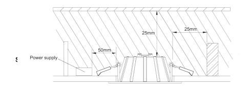
Rear of fitting may abut structural members and building elements. Do not install through or directly into joist, beam, rafter or ceiling batten.
