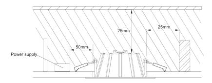
Rear of fitting may abut structural members and building elements. Do not install through or directly into joist, beam, rafter or ceiling batten.
