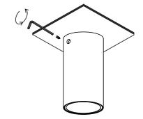
5 - Align the driver box to the counterpoint and rotate clock wise to fix onto the back base 6 - Lock base with grubb screw
