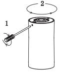
1 - Loosen the M3 screws Rotate the back base off the lamp anti-clock wise
