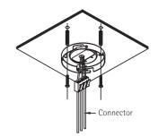
3 - Fix the back base on the ceiling by tapping screws
