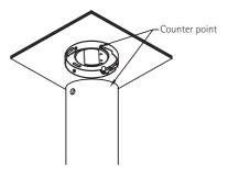
5 - Align the driver box to the counterpoint and rotate clock wise to fix onto the back base
