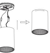
Fix the lamp and bracket by rotating clockwise.
