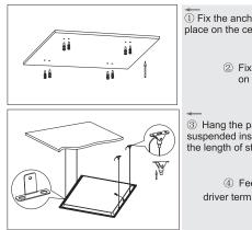
1) Fix the anchor into target place on the ceiling.
