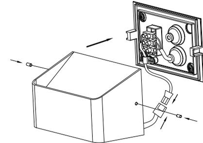
Get the lamp fixture back to the base and fix it well.
