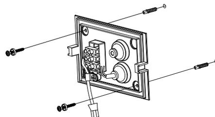
Fix the base on the wall and make the wires through the hole of the base.
