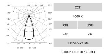
**GENERAL** High optical and energy efficiency recessed downlighter for accent illumination.
