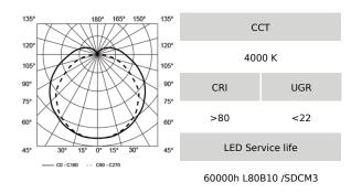
**GENERAL** Surface mounted luminaire for general illumination, with a simple, minimalistic shape.
