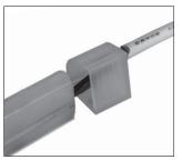
2. Push end of the wire through the power feed cap hole. Fill end cap with silicone glue and push onto end of UDON 1212. If attaching an end cap without a hole fill end cap with silicone glue and push onto the end of UDON 1212. Wait for silicone glue to cure.
