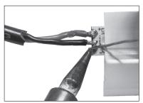
1. Solder on cable to solder pads inside UDON 1212. Make sure cable is firmly attached to solder pads.
