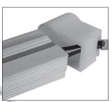
2. Push end of the wire through the power feed cap hole. Fill end cap with silicone glue and push onto end of UDON 1023. If attaching an end cap without a hole fill end cap with silicone glue and push onto the end of UDON 1023. Wait for silicone glue to cure.
