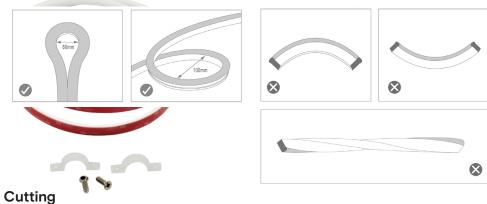
Cut UDON at the cutting mark (look through cutting window for the copper/dark spot and cut in the middle of this spot)
