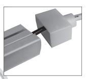
2. Push end of the wire through the power feed cap hole. Fill end cap with silicone glue and push onto end of UDON 1220. If attaching an end cap without a hole fill end cap with silicone glue and push onto the end of UDON 1220. Wait for silicone glue to cure
