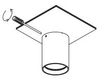
**F**. Align the front base to the counter point and rotate clockwise.
