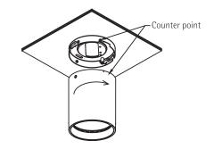
G. Tighten M3 screws. Completed installation.
