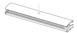
J. Turn on mains power supply and test luminaire for correct operation.
